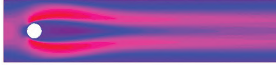
FIGURE 4.6 – Test 2 : The first component (along the x_1 -axis) of the steady-state velocity \mathbf{v}_s for R_e = 1000 .
